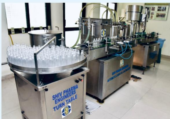
Liquid filling and cap sealing machine
