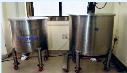
Cold process mixing unit for liquid formulations
